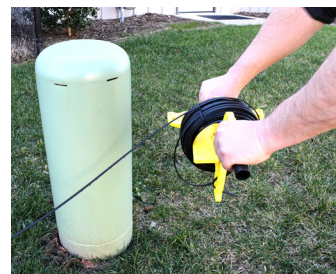
18-FFPC2: Fiber Driver, Hard Case, 14mm, 16mm, 18mm, 3/4in. & 1in. duct adapters)
